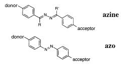
relevant to regiochemical issues in azine chemistry and they hold promise as novel NLO materials. Azines are closely related to azo compounds, a class of highly successful organic NLO materials, in that both diaza systems contain extended  $\pi$ systems with connected sp<sup>2</sup>-hybridized nitrogen atoms. The *crisscross* addition,<sup>2</sup> the tandem 1,3-dipolar cycloaddi-
