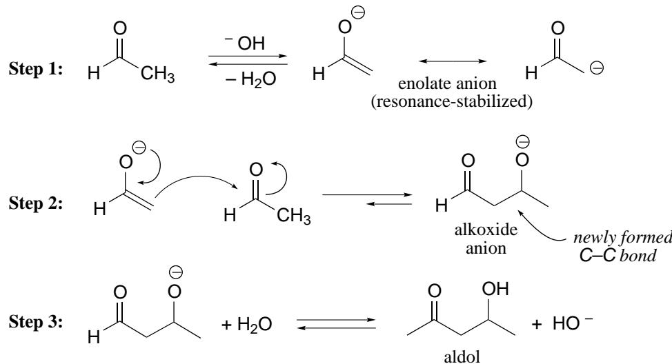
An aldol condensation between two different aldehydes or ketones is called a *crossed-aldol condensation*. Such condensations generally result in an undesirable mixture of products, although in some cases a single product may be obtained in good yield. An example of this is the crossed aldol condensation between acetone and benzaldehyde to give dibenzalacetone, which was carried out in past semesters of this course.
