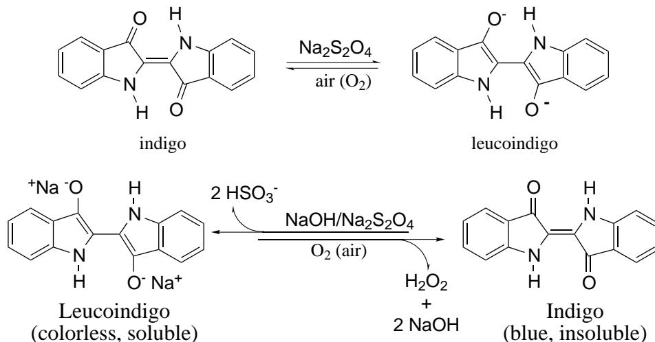
A solution of the leucoindigo is used to dye a piece of cloth. The cloth is then air-dried, which oxidizes the leucoindigo back to the indigo form. The cloth which you use is a small square of a special fabric called Multifiber Fabric 10, which has the following fibers woven into it: spun acetate rayon, cotton, a spun polyamide (Nylon 6,6), Dacron, Orlon, and wool.
