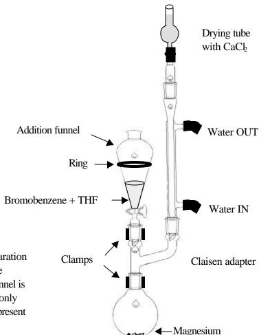
**Figure 1.** The apparatus for preparation of the Grignard reagent. During the flaming out process, the addition funnel is replaced with a glass stopper, and only the magnesium metal (no THF) is present in the flask.
