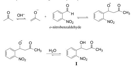
The hydroxy ketone (I) has been isolated and identified. In this experiment, however, it continues to react in a series of condensations, tautomerizations, a retro-Claisen condensation, and eliminations to produce indigo within a matter of seconds. The exact nature of these steps is unknown, and the scheme outlined below is pure speculation, although chemically plausible.
