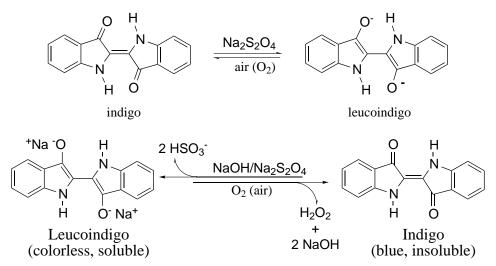
The blue, water-insoluble indigo is isolated and then treated with sodium dithionite, a reducing agent, to produce the pale yellow, water-soluble leucoindigo:
