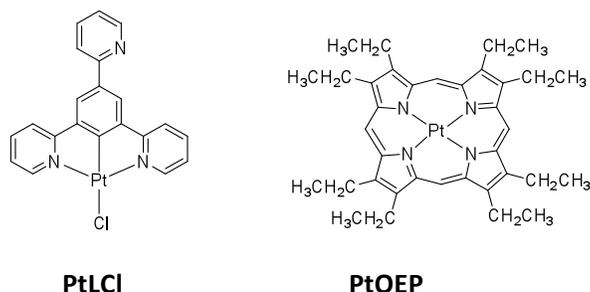
**Fig 1.** The chemical structure of O<sub>2</sub> sensor lumophores.
