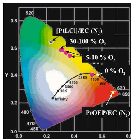
Fig. 3. CIE *xy* colour coordinates of the PtOEP/EC-PtLCl/EC dual-lumophore shows different sensor responses at different oxygen concentrations.
