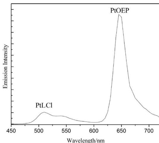
Fig. 2. Emission spectrum of PtOEP/EC-PtLCl/EC dual-lumophore sensors shows absorptions in the absence of oxygen at 295 K.
