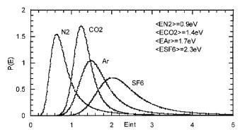
**FIGURE 11.** Internal energy distributions obtained for different collision gases for 15 V on the sampling cone (VG Platform instrument) and water/acetonitrile (50:50) as mobile phase. (Collette C, De Pauw E, Calibration of the internal energy distribution of ions produced by electrospray. Rapid Commun Mass Spectrom 12:165–170, Copyright © 1998 John Wiley and Sons. This material is used by permission of John Wiley and Sons.)
