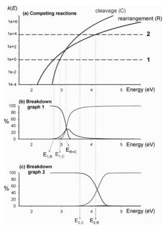
**FIGURE 2.** (a) Rate constants as a function of the internal energy for two hypothetical competing reaction channels (a rearrangement and a cleavage reaction). The curves have a RRKM-like dependency, but have been calculated with hypothetical critical energies and frequency sets. The breakdown diagrams for (b) instrument 1 ( $\tau = 10$  ms) and (c) instrument 2 ( $\tau = 1$   $\mu$ s) have been generated with Eqs. 3–6, using the hypothetical k(E) curves displayed in panel (a).
