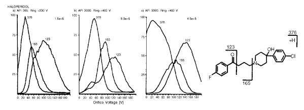
**FIGURE 4.** Chemical structure of haloperidol and breakdown curves from orifice ramping experiments using API 365 (a), API 2000 (b), and API 3000 (c) instruments. (Weinmann W, Stoertzel M, Vogt S, Svoboda M, Schreiber A, Tuning compounds for ESI/in-source CID and mass spectra library searching. J Mass Spectrom 36:1013–1023, Copyright © 2001 John Wiley and Sons. This material is used by permission of John Wiley and Sons.)
