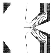
**FIGURE 8.** Geometry of the relevant part of the source of the VG Platform single quadrupole mass spectrometer as simulated by SIMION, equipotential lines, and one representative ion trajectory. (Reprinted with permission from J Phys Chem A 105, Hoxha et al., Mechanism of collisional heating in electrospray mass spectrometry: Ion trajectory calculations. pp 7326–7333, Copyright © 2001 American Chemical Society.)
